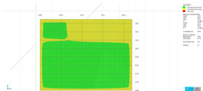
Touch and step voltages safe areas - Factory
