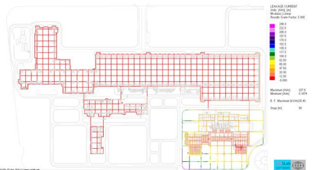
Leakage current - Large factory
